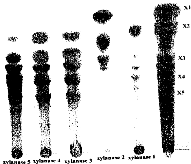
Fig. 5. TLC of hydrolysates of oat spelt xylan by the purified xylanases 1, 2, 3, 4 and 5
